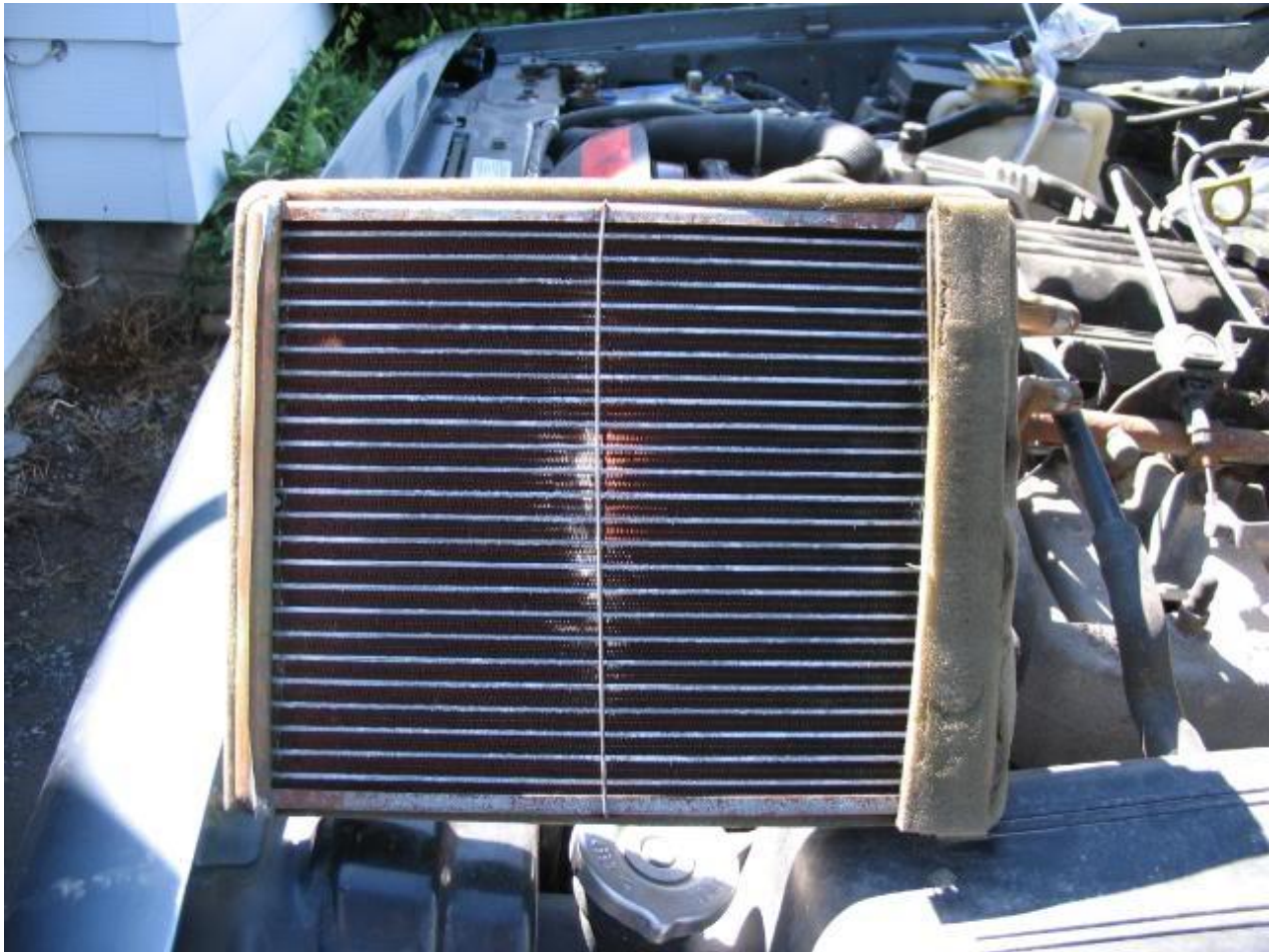
New heater core installed with foam (I used spray adhesive to stick the foam on the new cores)
