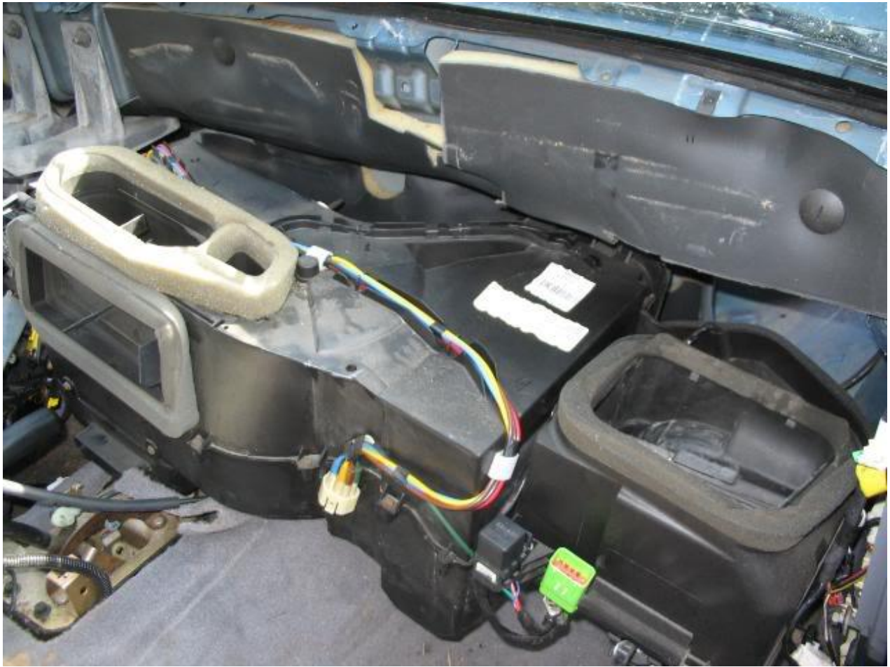
And this chunk of foam is what sat under the evaporator....nicely rotted away
