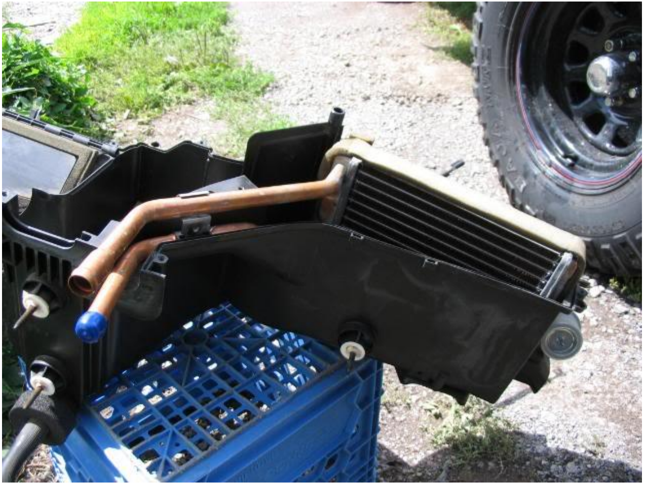
New Evaporator installed:
