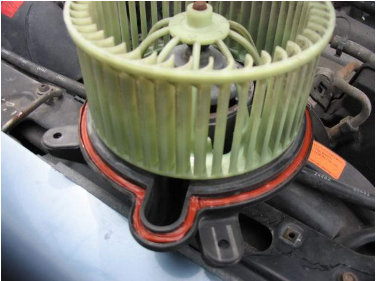
New foam seals installed on the HVAC box:
