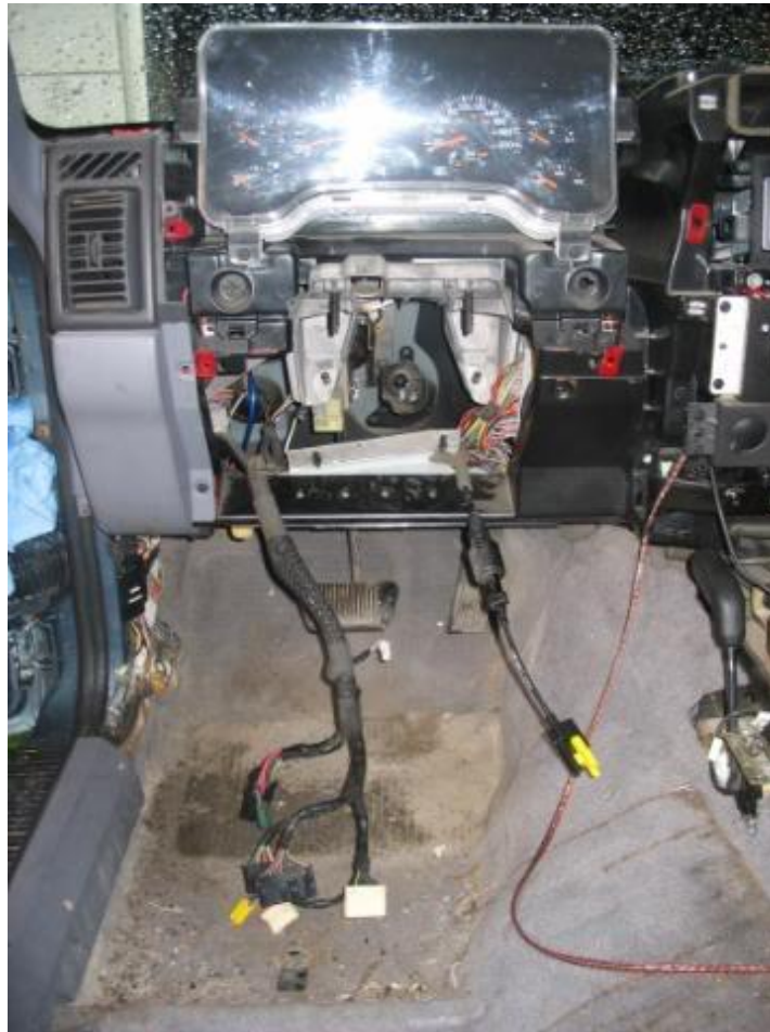
Here's a view of the mounting studs and coupler for the steering column:
