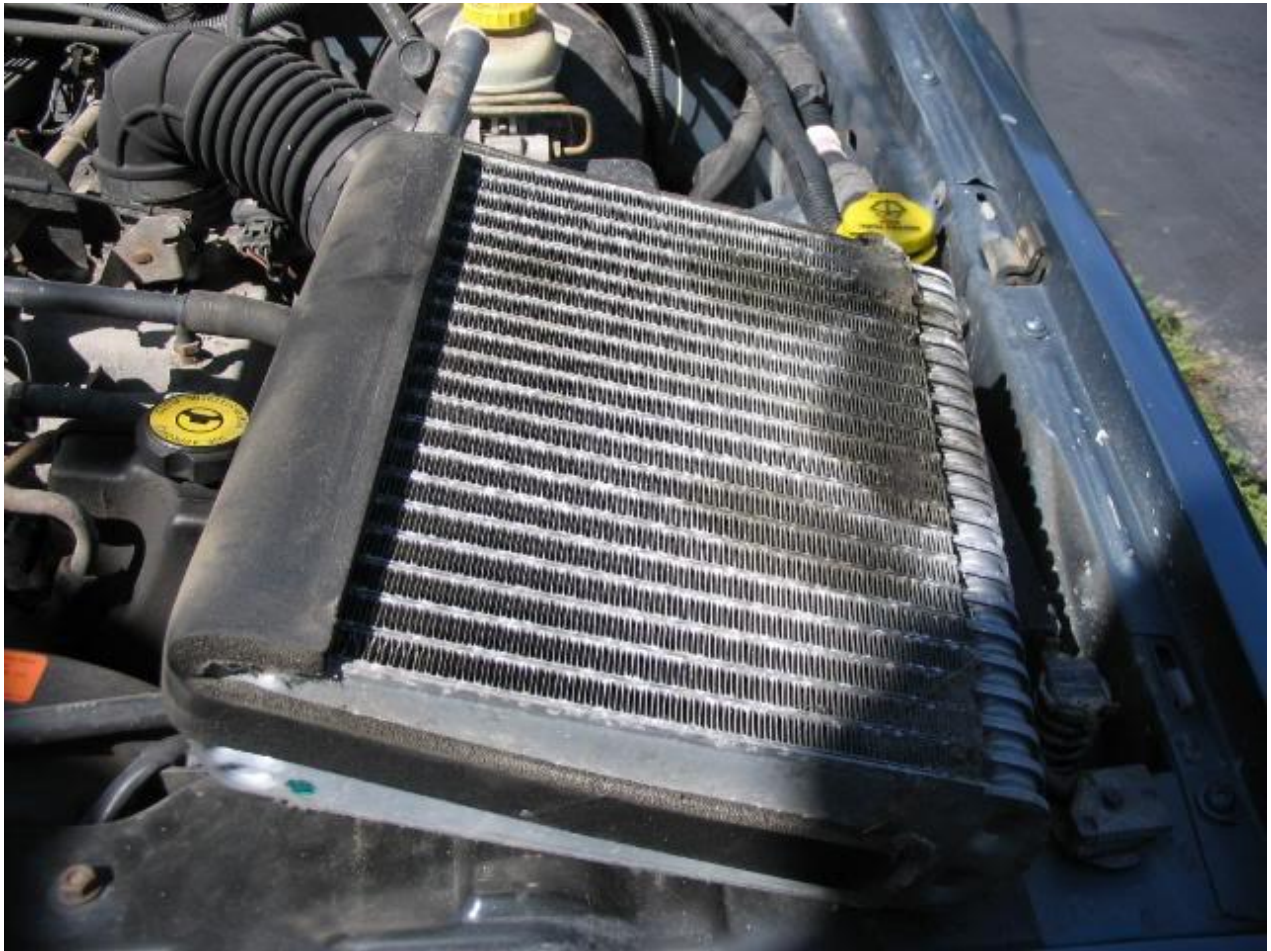
Ye Olde Heater Core (still works though)
