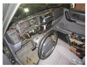
10) Remove kick panels (left and Right) and remove 2 dash mounting nuts. I removed the left vent cover to allow more room for the dash to swing out
