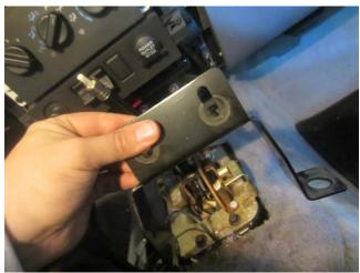
9) Drop steering column (2 nuts on left and right ) )
