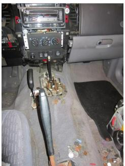
8) Remove bracket on tranny tunnel (4 nuts)
