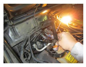
18) Disconnect vacuum line from t fitting.
