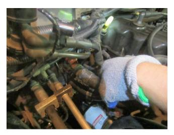
17) Detach evaporator tubes. First pop guards off by pulling up and remover condesor from the bracket (it is attached to 2 of the bolts holding the hvac to the firewall). Use the propper disconnect tools by clicking them in from the back. (I
