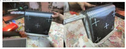
The OEM heater core was clearly shot. My project was delayed because the OMIX ADA replacement core had a bad fit . . . too big and tubes not exact. I might have been able to make it work without insulation, but found a Spectra Premium (seen next to Oem) locally. Pretty close as far as fit is concerned and it came with foam.
