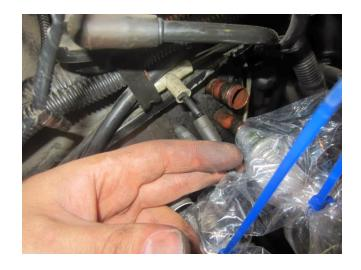
19) Remove remaining three nuts from the firewall. The one in back of the head IS a PITA. A snap and wire harness hanger must first be removed and then you should be able to get a 11mm or 7/16 box wrench on it. (Note: it helps to pb blast these bolts ahead of time and use offset ratcheting box wrench)
