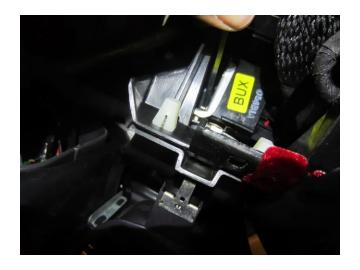
4) Remove Shroud . . . several screws around shroud, disconnect collar around
