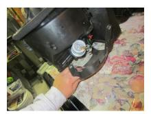
The insulation around the blower motor can be cut with a blade where the box separates. I patched it with insulation glue upon reassembly. The foam around the must be gently peeled off with a scrapper if you plan to reuse . . . I patched mine up a bit and glued it back.
