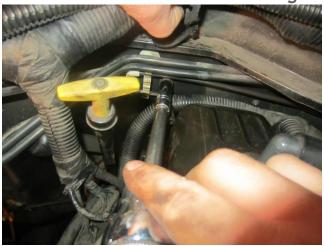
20) Back in the vehicle, disconnect wire harness that passes through HVAC box on the far right. Luckily I saw this before I ripped the box out.
