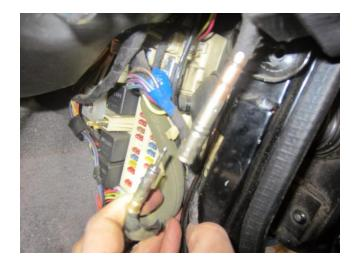
13) Disconnect bled door cable from HVAC. This was actually one of the hardest parts for me. With cold and brittle parts, I needed to take apart a lot of the parts in the HVAC control box to get the cable out.
