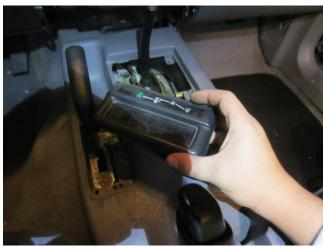
7) Unscrew center console (by shifter and transfer case lever) and remove.
