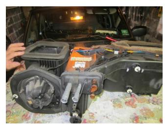
22) Open up box (many 8 mm bolts + removal or separating of insulation, and disconnecting vac lines and plug) and replace parts. See this detailed writeup for a more in-depth look at how to do all work on the actual HVAC box: http://www.scribd.com/doc/176480289/Jeep-XJ-Heater-Core-and-Evaporator-Replacement
